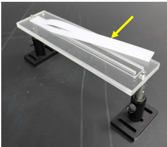
Figure 7: Modified acrylic design featuring two pieces of clear acrylic drilled with continuous slots of varying sizes. The arrow points to a strip of silicone rubber. The table shows the parts that were used to construct the acrylic support template
